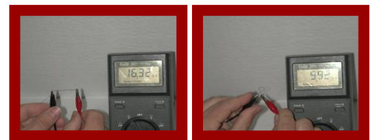
Figure 2. Photos demonstrating electrical properties of PPy-coated Gütermann cotton thread.
